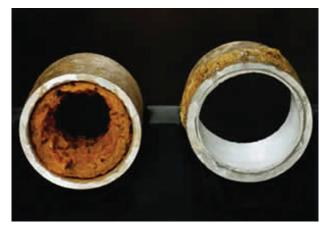
In the above the pipe on the left is the build-up of organic matter which occurs over time. With the correct dosing of the Drain Odour Eliminator & Maintainer the build-up of the organic matter is removed. As you can see the drain pipe then becomes free flowing. As the build-up in the pipe increases the urine and any liquid builds up behind the build-up, this then causes odours to go back up the pipe into the bathroom or building.
