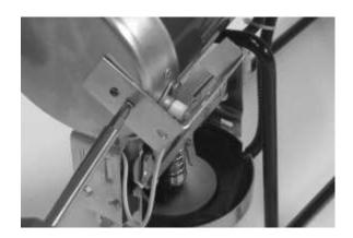
2. Manually trigger the cannon's firing mechanism by lifting up on the firing lever and releasing it so it hits the igniter. Look for a spark between the electrodes on the spark plug.
